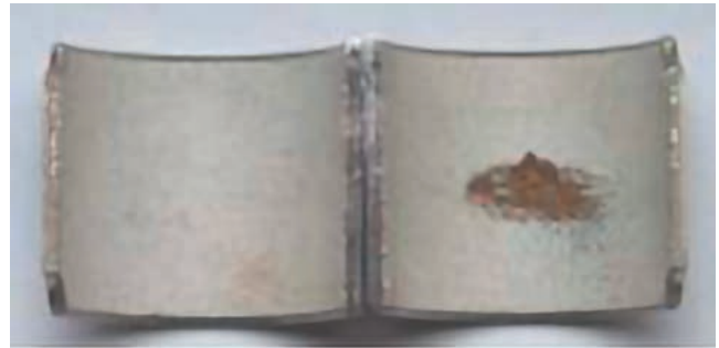
Fig. 36: Local damage caused by cavitation
