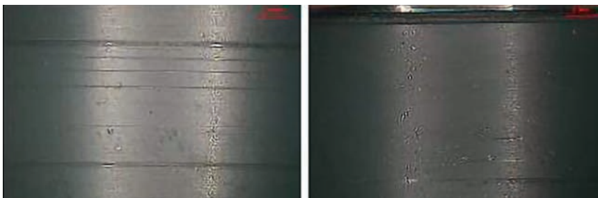
Fig. 38: P2 plain bearing, grooves in the sliding surface
