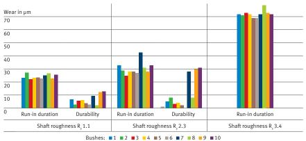
Analysis rotating test bench: Wear in  $\mu m$  with different shaft roughness  $R_z,$  shaft hardness HRC 60
