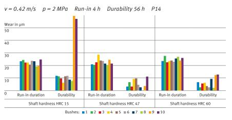
Analysis rotating test bench: Wear in µm with different shaft hardness HRC
